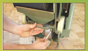
Remember, as you are looking at the underside of the machine; the further the wheel away from you, the heavier it will sand on that side. Only one wheel is adjustable, and it is marked with a rudimentary black arrow.
